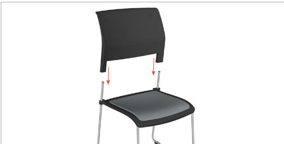
STEP 5: Position back shell on chair frame.
