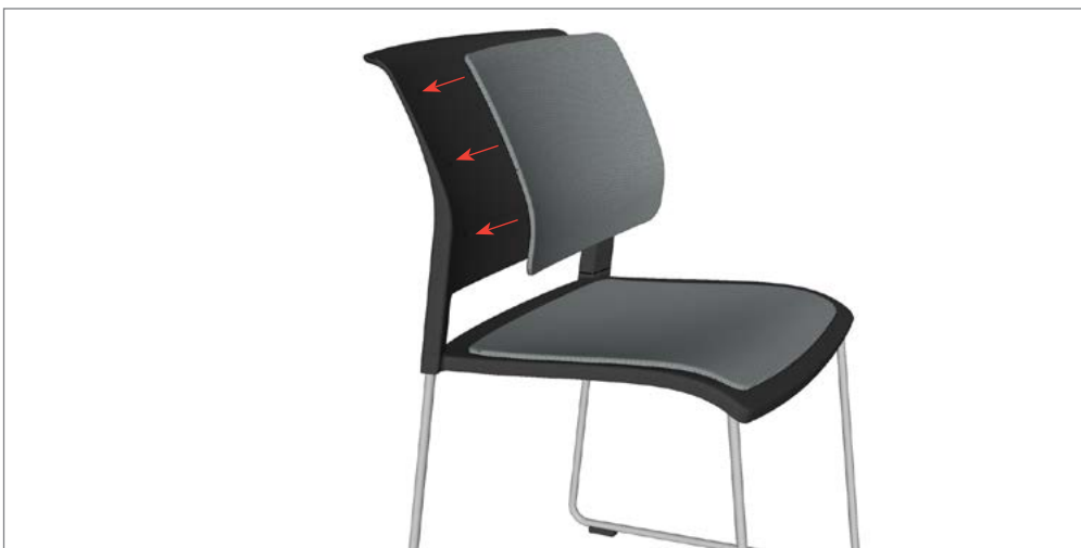
STEP 7: Attached back pad into back shell.
